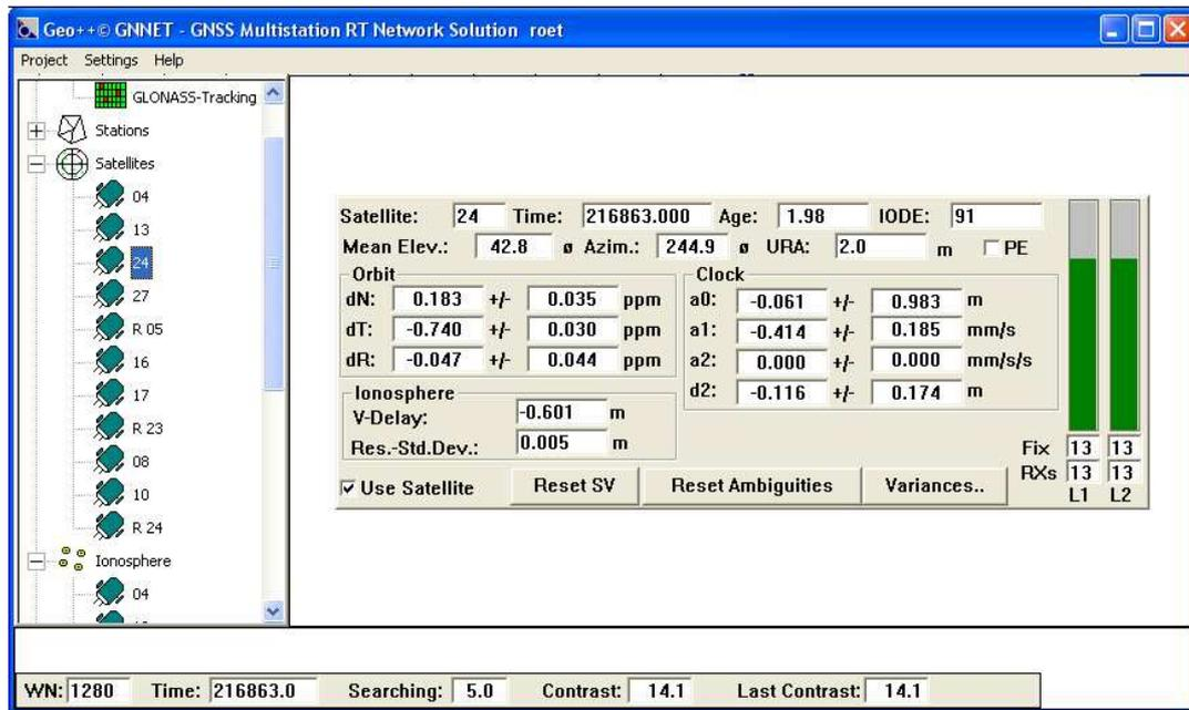
Fig. 2: GNSMART GNNET window with current estimate of satellite dependent functional models
