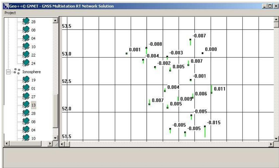
Fig. 3: GNSMART GNET window with current estimate of stochastic ionospheric model of PRN 13
