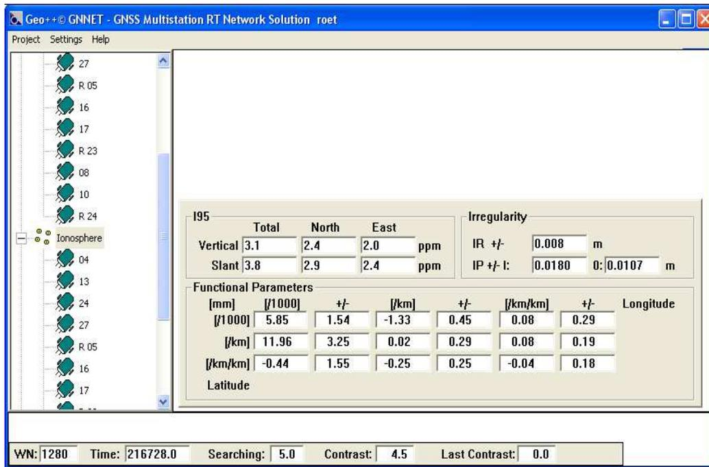
Fig. 1: GNSMART GNNET window with currently applied functional ionospheric model and currently computed ionospheric indicators (irregularities and I<sub>95</sub> index)
