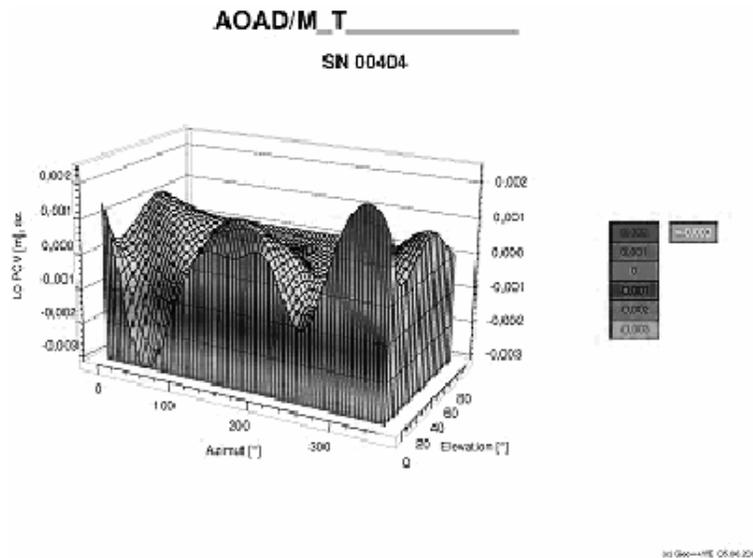
Azimuthal PCV L0 (offset and elevation dependent terms removed)
