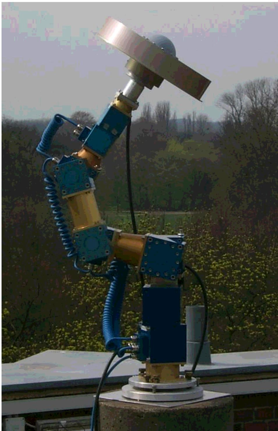
(original AOAD/M\_T Choke Ring antenna on the robot during calibration procedure)
