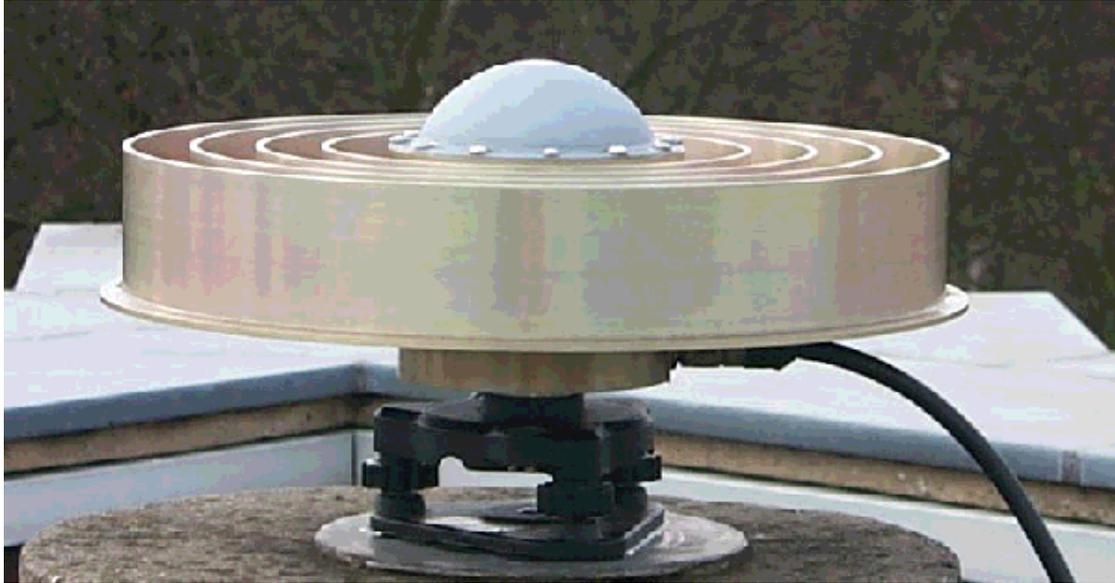
(original AOAD/M\_T Choke Ring antenna used for this calibration)
